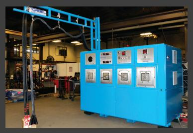
Nexjen Electric Motor Test Systems are built on the principle of safe, simple operation and dependable service. The same Jenkins test transformer design we have used for the past fifty years sits at the core of a power supply engineered to perform continuously at full ratings for 8 hours. With heavy duty components and very few moving parts, the Nexjen Electric Motor Test System is designed to operate for decades without maintenance.
